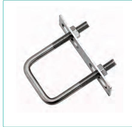
U Shaped Bolt Material: Carbon Steel / SS Surface: Zinc / Customized Size: Φ22, Φ25, Φ32
